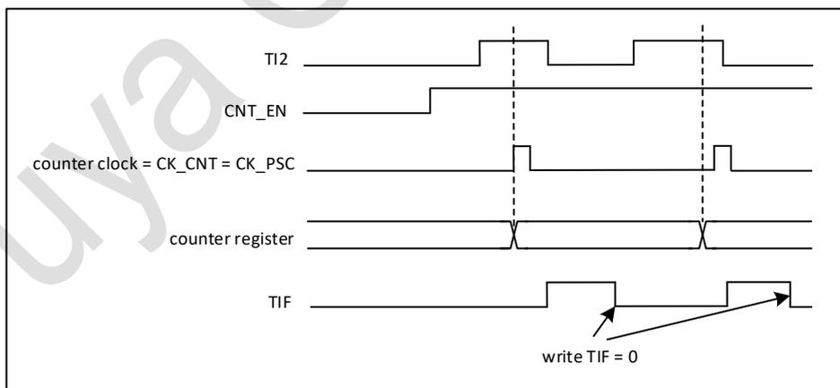
图 18-23 Control circuit in external clock mode 1
