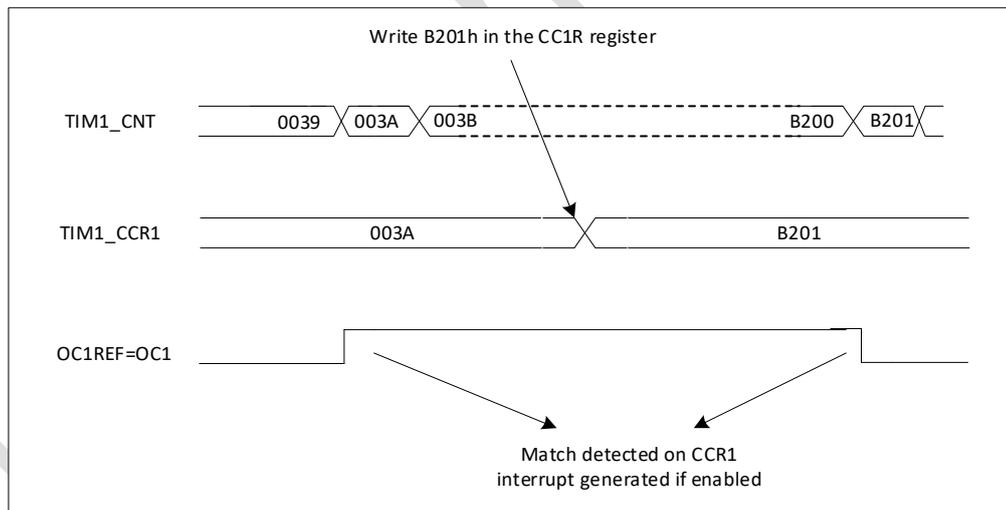
图 20-15 Output compare mode, toggle on OC1
